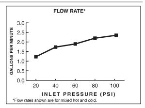
2.2 gpm/8.3 L/min. FLOW RATE
