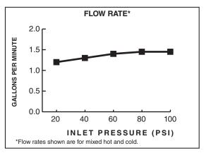
1.5 gpm/5.7 L/min. FLOW RATE
